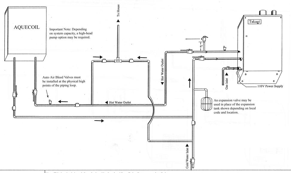
This diagram is provided as a curtesy by Takagi USA and has been modified by
